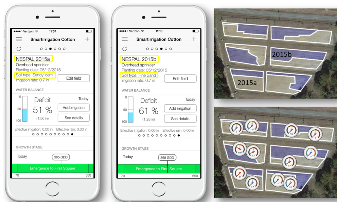
Fig. 11. The research field at the right was delineated into two IMZs (2015a and 2015b) using soil electrical conductivity as a surrogate for soil texture. The two IMZs were registered as individual fields and the RZSWDs for each IMZ were used to create VRI prescription maps when irrigation was needed. Each IMZ received a different irrigation amount from the field's VRI-enabled pivot. The gages in the field indicate location of UGA SSA sensor node locations. The two different RZSWDs are the result of differences in soil texture between the IMZs.
