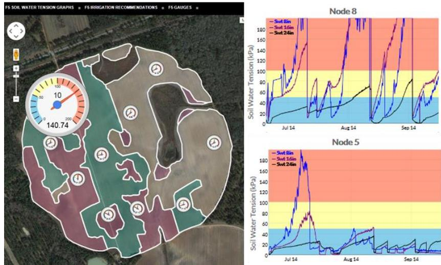
**Fig 4. Two different visualizations of UGA SSA soil moisture data. On the left is current soil water tension displayed through color-coded gages. Touching the gages with the cursor or finger enlarges them. On the right are soil water tension curves for the entire growing season. Note the dramatic difference in response between two nodes in the same field.**
