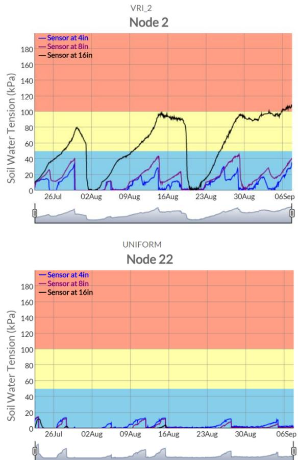
**Fig 8. Season-long soil moisture data graphs from the VRI strip (top) and Uniform strip (bottom). The soil in the uniform strips is being maintained much wetter than in the VRI strips.**
