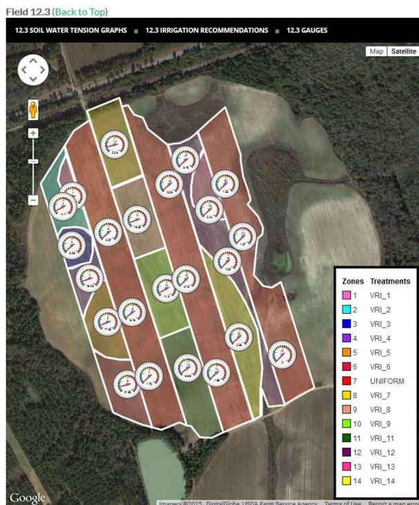
Fig 6. VRI Zones and field used for the 2015 on-farm VRI evaluation of dynamic VRI. The gages indicate the location of UGA SSA sensor nodes.
