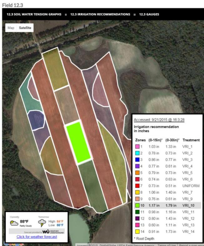
**Fig 7. Dynamically developed irrigation scheduling recommendations for each IMZ. Clicking on either the zone or the recommendation will highlight both. In the figure, zone 10 is highlighted. The recommendations are to bring the soil profile to within 75% of field capacity.**
