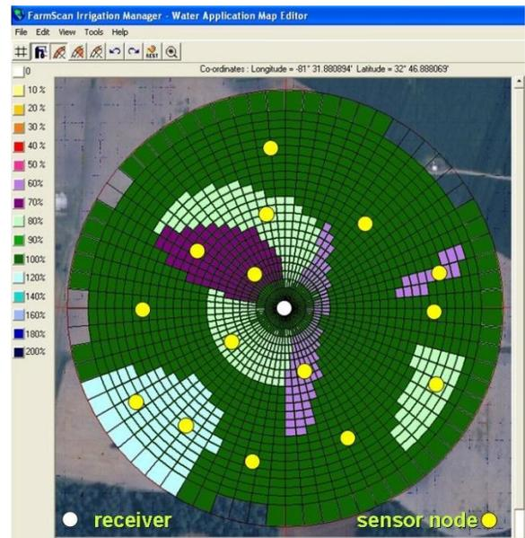
Fig 2. VRI prescription map for a 51ha field in Georgia. Grids represent discreet areas which can receive unique application rates. The yellow circles represent potential locations of soil moisture sensor nodes.
