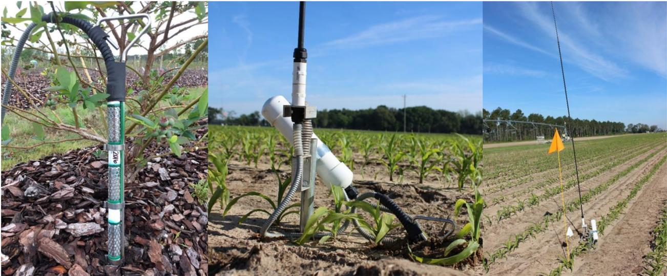
**Fig 3.** A UGA SSA sensor node has a low profile when installed in the field. The flexible whip antenna allows field vehicles to pass directly over the node.
